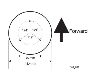
Mounting: Drill 3 x Holes (size depends on the material being drilled)
